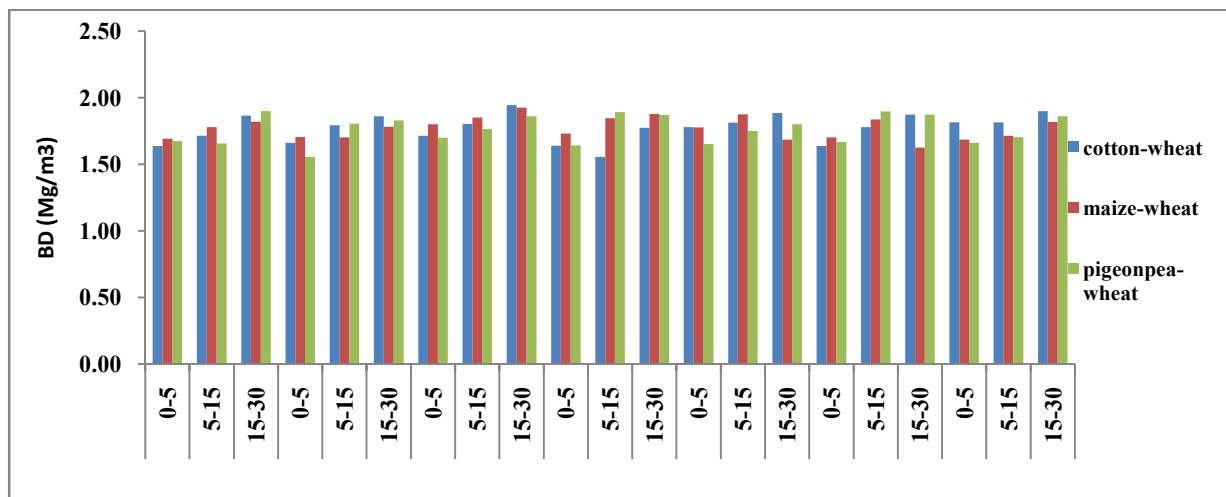
Fig. 3. Bulk density of soil as influenced by conventional and conservation agriculture practices in cotton-wheat, maize-wheat and pigeon pea-wheat system
